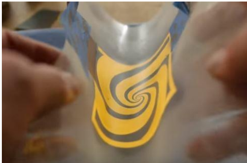
Figure 4 EL paint display on flexible substrate
